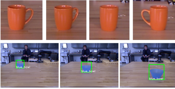
Fig. 2. Top row : Example data captured using our object localization procedure with multiple orientations. Bottom row : Example output of object detection pipeline with multiple positions.
