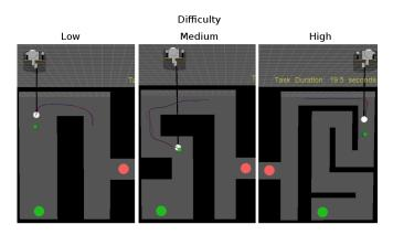
Fig. 2. Example maze environments for the simulated planar crane task, showing initial position (red circle), target position (green circle), current position of the user input (smaller green sphere), reference trajectory (blue line), executed trajectory (red line), suspended mass (white circle), and maze walls (black). A robotic winch (grey) manipulates the location and length of the string supporting the payload.
