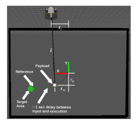
Fig. 1. Definition of the system configuration variables  $x_m$ ,  $y_m$ ,  $x_r$  and l. The delay between user input (green line) and execution (blue line) is approximately 1 second.
