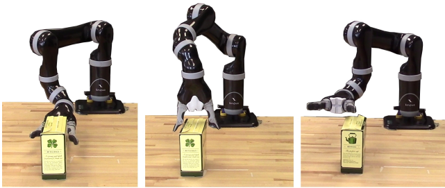
Figure 7. Example experimental result of ambiguous input from a user that resulted in a grounding different from the user’s true desire. In the initial trajectory the arm tries to pick the box up on the side (left). In the desired correction the arm should pick the box up from the top (middle). Instead, the correction provided by the user (“over”) resulted in the arm moving above the box without trying to grasp it (right).
